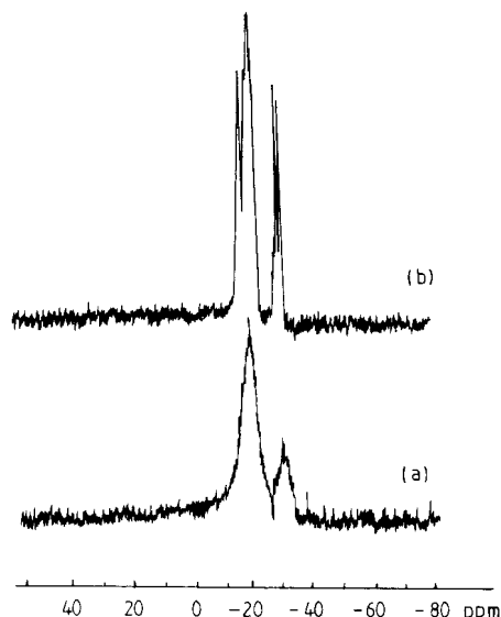
Figure 3 ^{29}\text{Si} NMR spectra of (a) polyaluminasilazanes 7–10 and (b) oligomethylsilazane [\text{CH}_3\text{Si}(\text{H})\text{NH}]_n .
